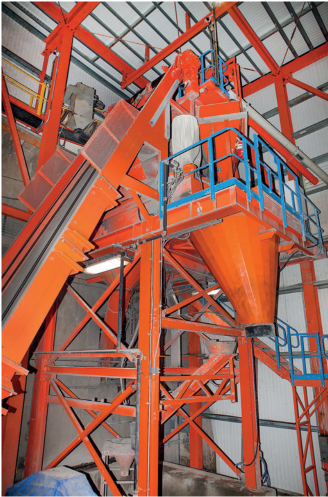
Figure 10: The view from below the mixer platform holding the ACT/Wiggert HPGM 4500 planetary countercurrent pan mixer.
