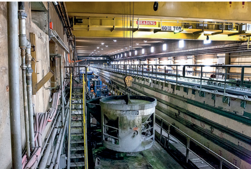
Figure 15: Concrete buckets suspended from a bridge crane are in continuous motion to supply Northeast Prestressed Products production facility in Cressona, Pennsylvania, USA.
